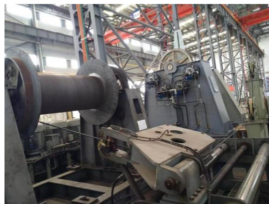
图 9 电缆收放试验设备 Fig.9 Cable retraction experiment equipment
