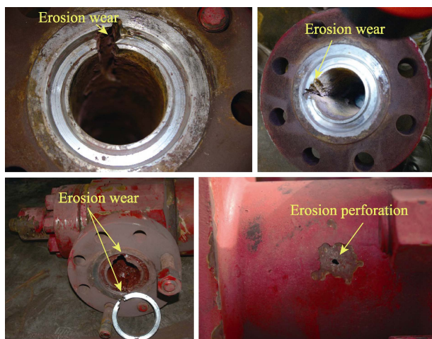
图 1 常见的冲蚀磨损现象 Fig.1 Common erosion wear phenomenon
