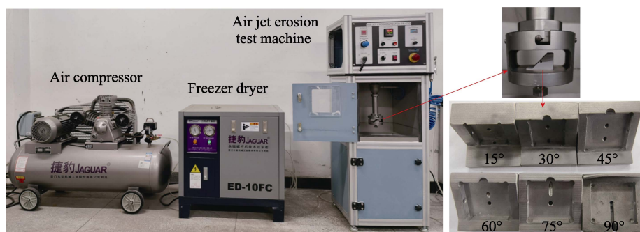
图 2 空气射流实验装置及试样支架 Fig.2 Air jet test device and sample support
