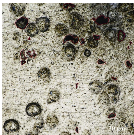
图9 加入微磨粒后的钛钽合金表面 Fig.9 Ti-Ta alloy surface after addition of micro-abrasives
