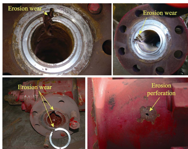
图 1 节流管汇的冲蚀磨损 Fig.1 Erosion morphology of choke manifold
