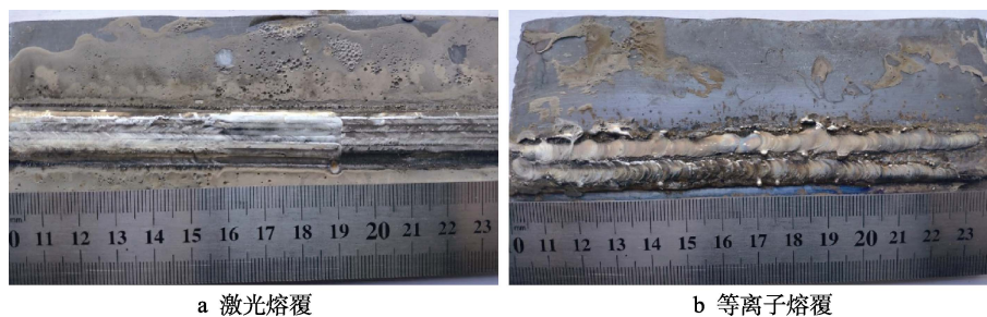
图 1 熔覆试样宏观形貌 Fig.1 Macro morphology of cladding sample: a) laser cladding coating; b) plasma cladding coating
