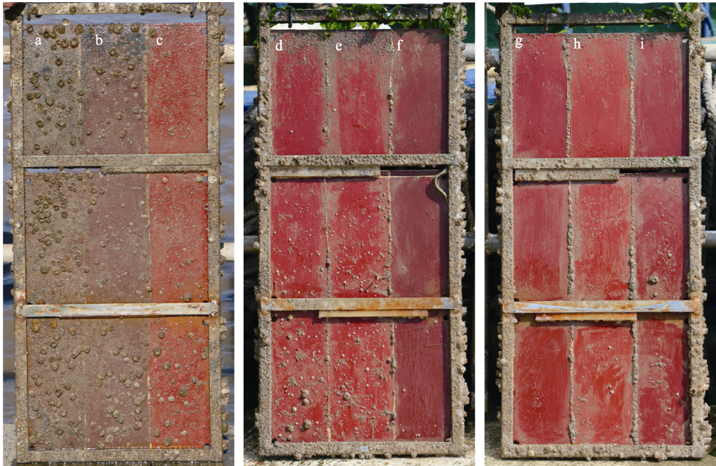
图 6 防污涂料浅海浸泡实验照片 Fig.6 Pictures of anti-fouling test in shallow submergence
