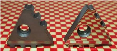
图 8 硬质合金刀片前刀面抛光前后对比 Fig.8 Comparison of rake surface of cemented carbide inserts before and after polishing
