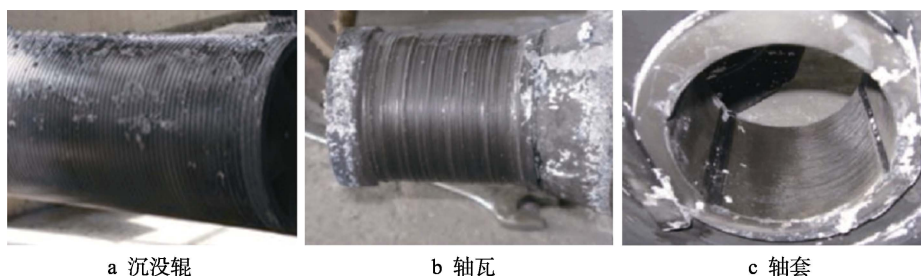
图 7 腐蚀及磨损失效实物图 [31] Fig.7 Failure of corrosion and wear [31] : a) sink roll, b) sleeve, c) bush
