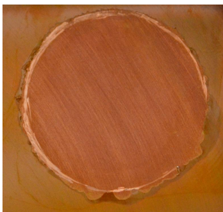
图10 聚酰亚胺涂层附着力测试的断面形状 Fig.10 Section shape in polyimide coating adhesion test
