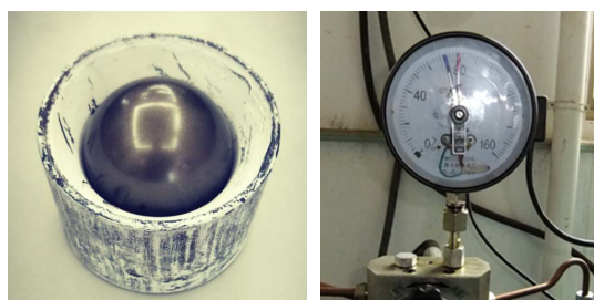
图15 4号球座承压密封测试 Fig.15 No.4 ball seat pressure sealing test
