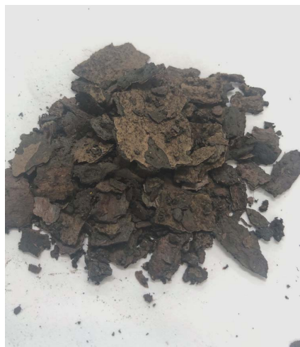
图 10 内壁腐蚀产物 Fig.10 Corrosion products of inner wall
