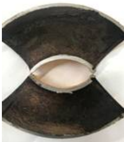
图 2 弯头内壁腐蚀形貌 Fig.2 Corrosion morphology of inner wall of elbow
