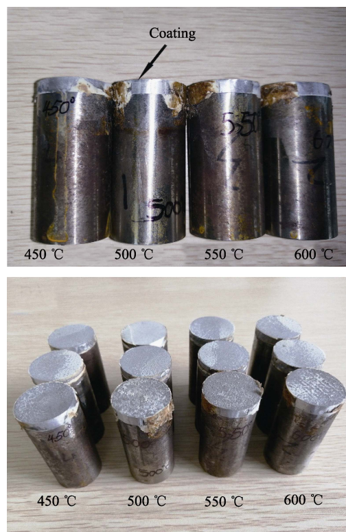
图 8 结合强度测试试样失效模式 Fig.8 Failure mode of samples in bonding strength test
