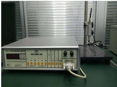
图 1 双电测四探针电阻仪 Fig.1 Double electric four-probe tester
