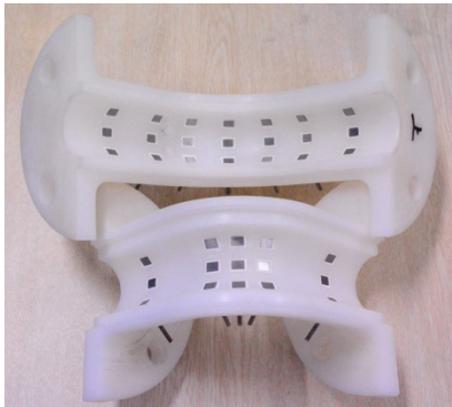
图 2 测试弯管及试样安装图 Fig.2 Installation diagram of the test bend and sample
