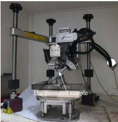
图 7 残余应力测量仪器及试样 Fig.7 Measuring apparatus of residual stress and the measured samples
