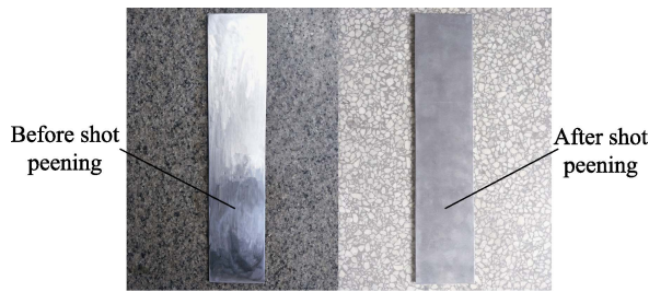
图 9 喷丸前后实验试样 Fig.9 Experimental sample before and after SP
