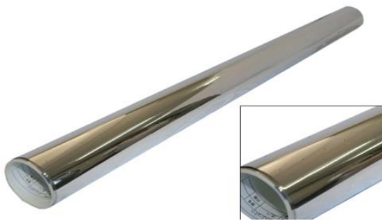
图 1 大面积双面镀铝聚酯薄膜 Fig.1 Large area of double-sided aluminized polyester film
