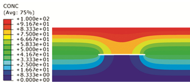
图 5 无应力场作用时氢浓度云图 Fig.5 Contour plot of hydrogen concentration without stress field
