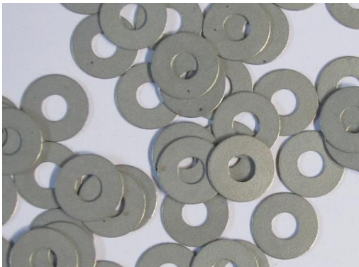
图 1 机械镀锌垫片外观 Fig.1 Surface of the washer deposited by mechanical plating
