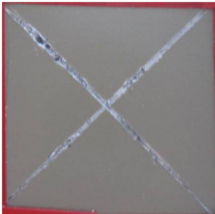
图 4 涂层试样 Machu 试验 120 h 后表面形貌 Fig.4 The surface morphology of the coated sample Machu tested after 120 h
