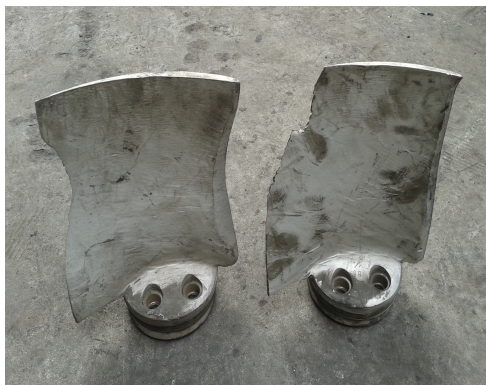
图 1 一次风机叶片磨损后的状态 Fig.1 Worn state of primary fan blades
