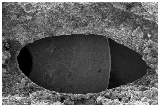
图 4 穿孔显微形貌 (10×) Fig.4 Morphology of perforation
