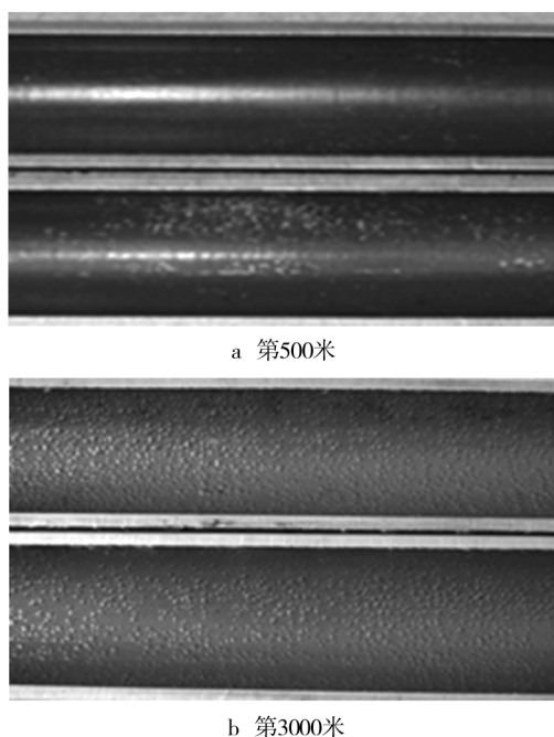
图5 G4x-x井第500米和第3000米油管剖开后内涂层对比 Fig.5 Comparison of internal coating of oil pipe at 500 meters and 3000 meters in well G4x-x
