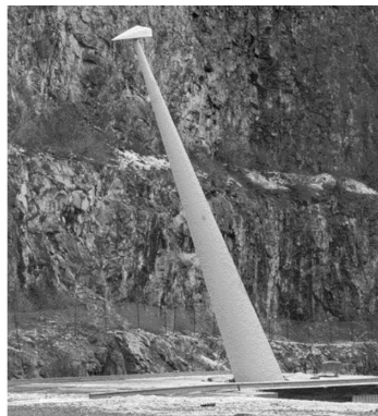
图 4 Underwood Quarry 测试场的椭圆型金属支架 Fig. 4 The oval melt support of Underwood Quarry
