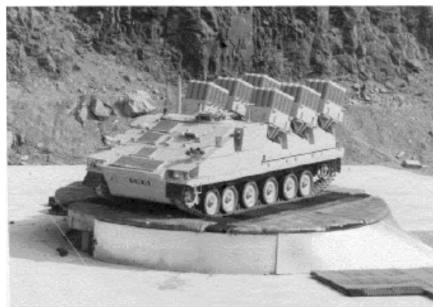
图 5 Thales Underwood Quarry 测试场开展的坦克 RCS 测量 Fig. 5 RCS measurement for tank in Thales Quarry measurement range
